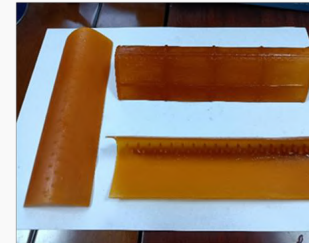
Shaped thin-walled complex antenna substrates
