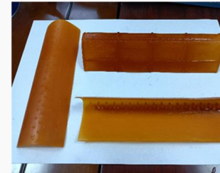
Shaped thin-walled complex antenna substrates
